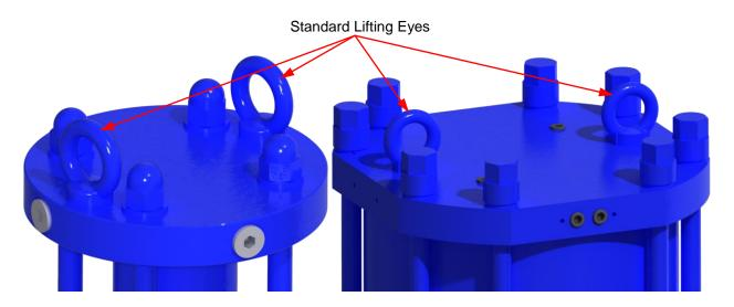
The below image is the standard lifting label attached to all SRC/SRC & DA actuators. **Do not use lifting** eyes to lift actuator and valve together as lifting eyes are only rated for the valve actuator only.
